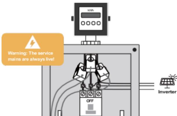
4. Insert each 3.5mm audio plug of Main CT into the corresponding audio jack on the top of the Energy Monitor:
