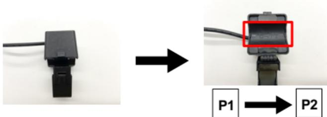
2. Clamp each Sub CTs around the circuit you wish to monitor. **Make sure the arrow on the CT must point towards the load or inverter!**
