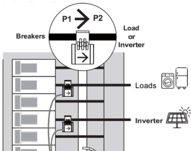
**Note:** If the circuit you are monitoring can generate energy such as Inverter, etc., after all the wiring is completed, please manually set the phase of the circuit in the app settings, otherwise the power measurement will be incorrect.
