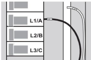
If your system is 3-Phase, secure the L2, L3 wire corresponding to L2/B, L3/C breaker pole.
