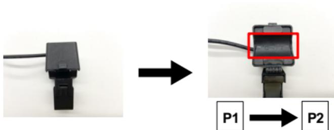
2. Clamp one Main CT on each main service lines. ***Make sure the arrow on the CT must point towards the breakers!*** Your system may have 1, 2, or 3 main service lines, and a corresponding number of Main CTs are required.
