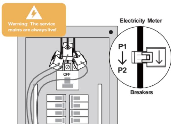
3. If you have Line/Service-side tap solar, Main CT must be clamped between the electricity meter and incoming feeds from inverter.
