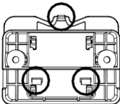
Locate the hooks of the mounting bracket and line up the hooks with the mounting holes on the Energy Monitor. Fit the hooks into the mounting holes as the picture below. Installation is now completed.
